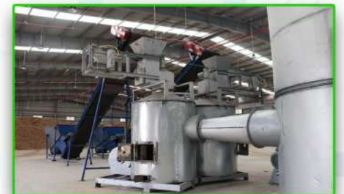
Wood chip burner
